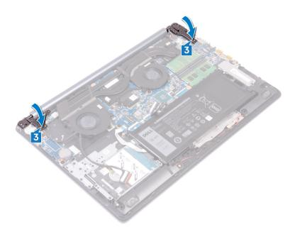
4 Replace the six screws (M2.5x6) that secure the left and right hinges to the system board and palm rest and keyboard assembly.
