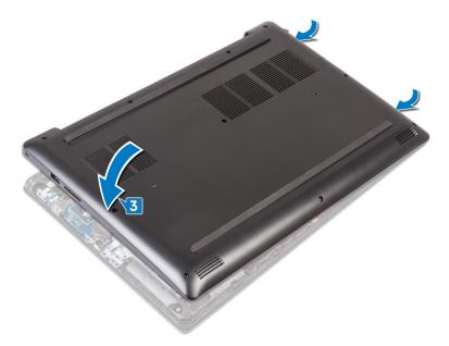
4 Align the tabs on the base cover with the slots on the palm-rest assembly and snap it into place.
